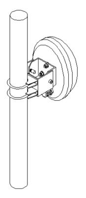
Fig. 3 Installation of transmitter/receiver on pole
