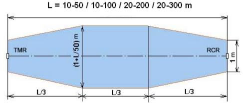
Fig. 2 Approximate clear zone shape for Radon - 50/ 100/ 200/ 300
