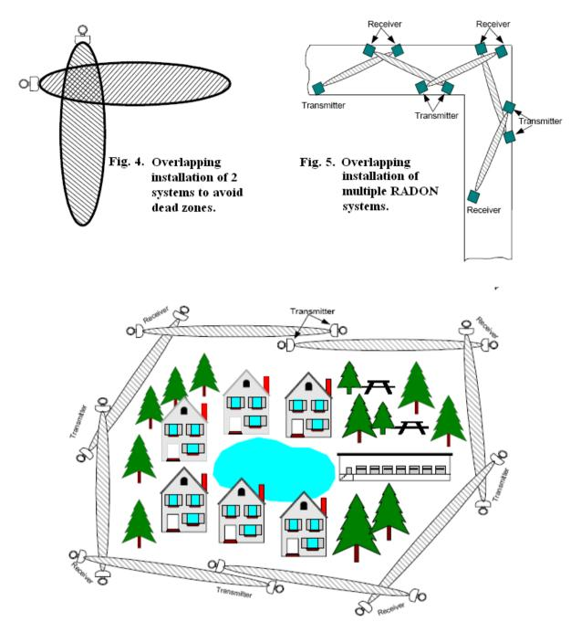
Fig. 6 Overlapping installation of RADON systems for perimeter protection
