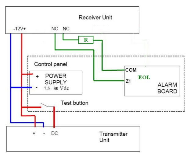
Fig. 9 Connection to alarm control panel
